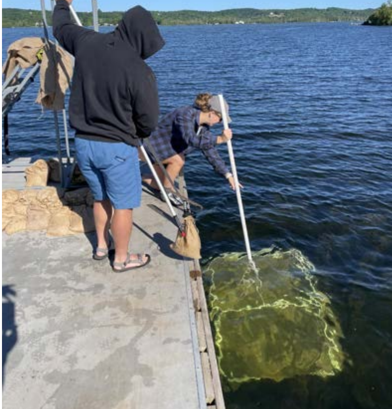
Figure 8 – Innovative Shallow Water Burlap Application Device
